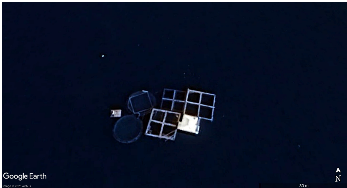
Figure 4. Examples of aquaculture gears used by local community in Puerto Princesa, Palawan identified in Google Earth images. The size of gears varies from 12 to 40 meters.
